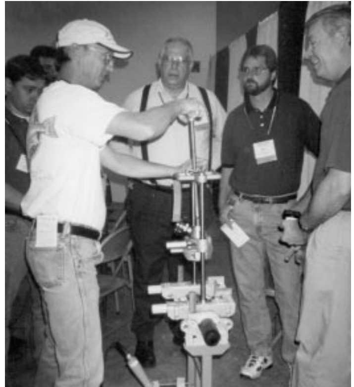
Students are hands-on testing with the McElroy Sidewinder™ (above) and the No. 28 Fusion (at left) machines.
